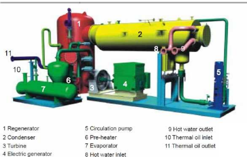
Figure 34. Organic Rankine Cycle scheme
