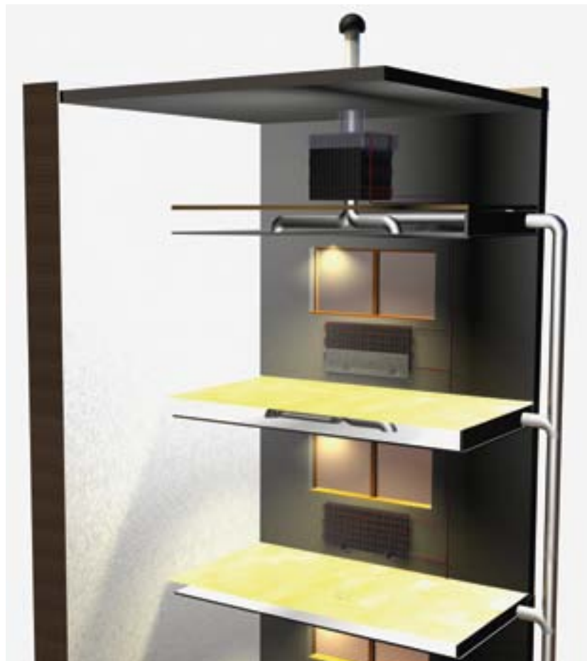
Façade-integrated natural ventilation system with heat recovery.
